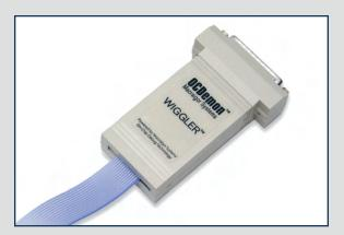
The Wiggler is a low cost interface used in the design, debug, and programming of microprocessor and microcontroller-based embedded systems. One side of the Wiggler interfaces to the parallel port of a host PC and the other side connects to an OCD (On-Chip Debug) port on the target system. As with all Macraigor interface devices, the Wiggler can simultaneously debug up to 255 devices on a single scan chain.
